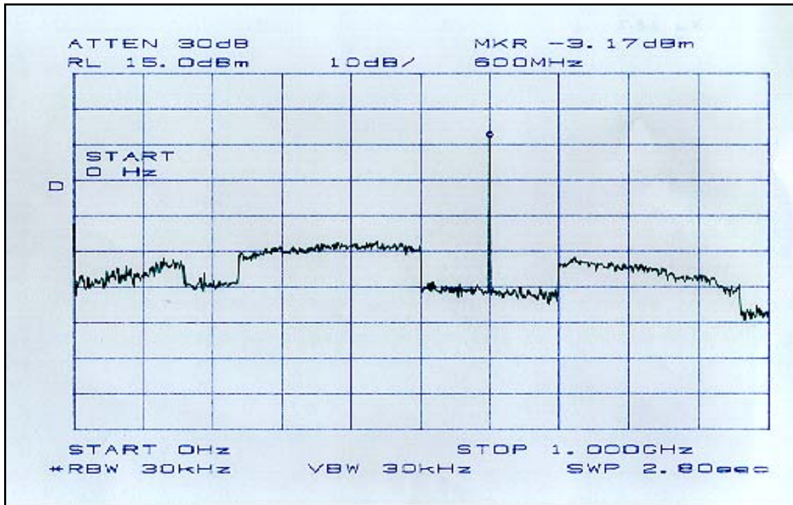
Figure 3.8.2 Spectrum of photodetected signal as seen on the spectrum analyzer.
