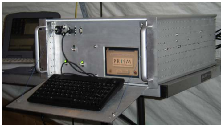
Figure 6.1: 8-Channel integrated Iridium communication system.
