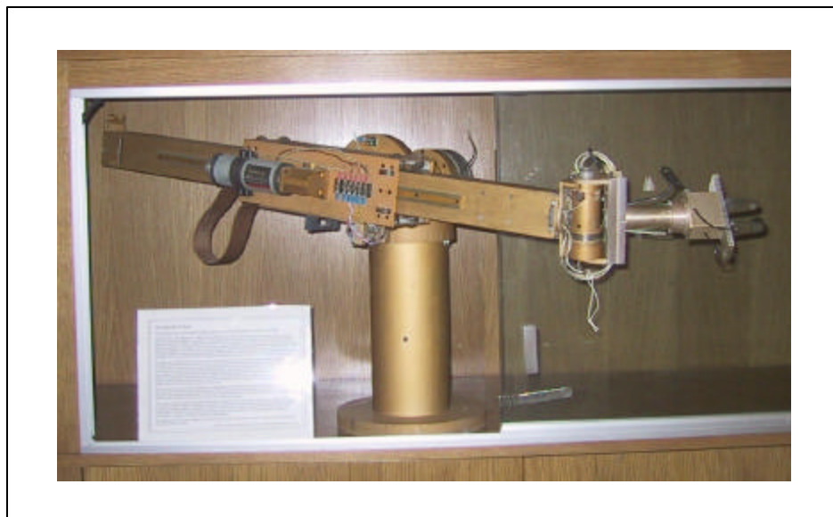
Figure 1. The Stanford/Rancho Arm (Rahman et al. , 2000).
