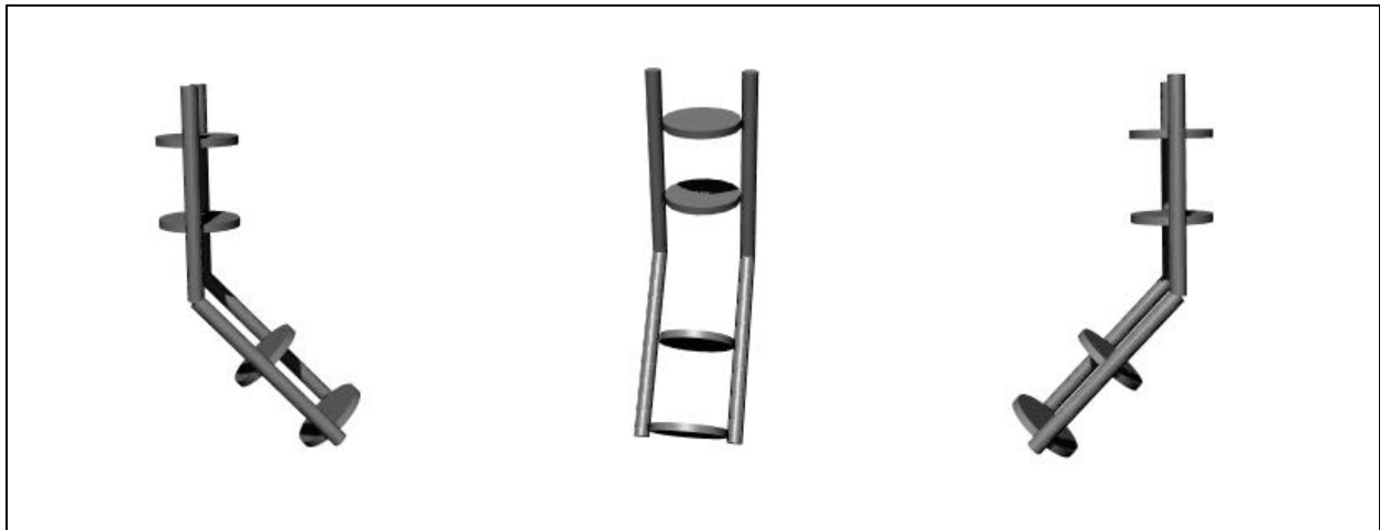
Figure 3. Base design of orthotic exoskeleton (the circular rings will have one large hole in the middle of each circle for arm, this was not possible due to software limitations).
