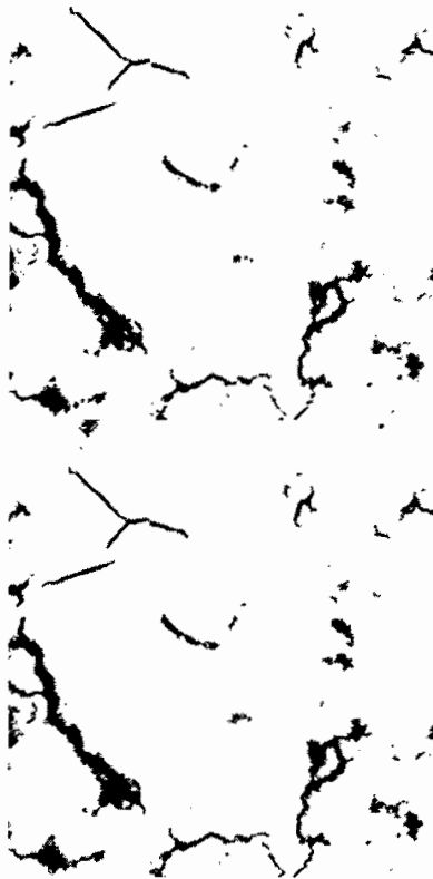
Fig. 12 Experiments on connecting objects. The raw image shows a photo of cement with cracks and other composites. The middle column shows the thresholded result. As observed, cracks (dark linear structures) were broken. By restricted growing the objects (bright regions), we increased dark regions. As a result, cracks were substantiated and connected, as shown in the right column. This allows a more accurate geometric analysis of the cracks.
