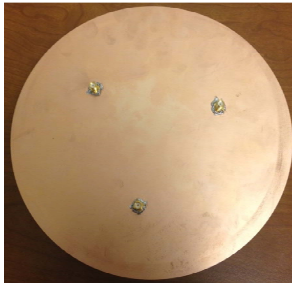
Fig. 4.2: Bottom view of final monopole array showing the three SMA connectors.
